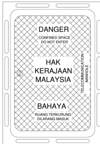
Figure 5.3 : Typical manhole cover using concrete
